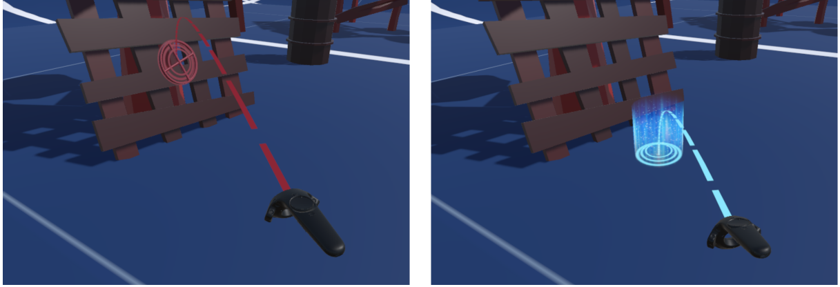
Figure 3.2: The color of teleportation curve was changed from blue to red when the teleportation path was interrupted by one of the objects.
