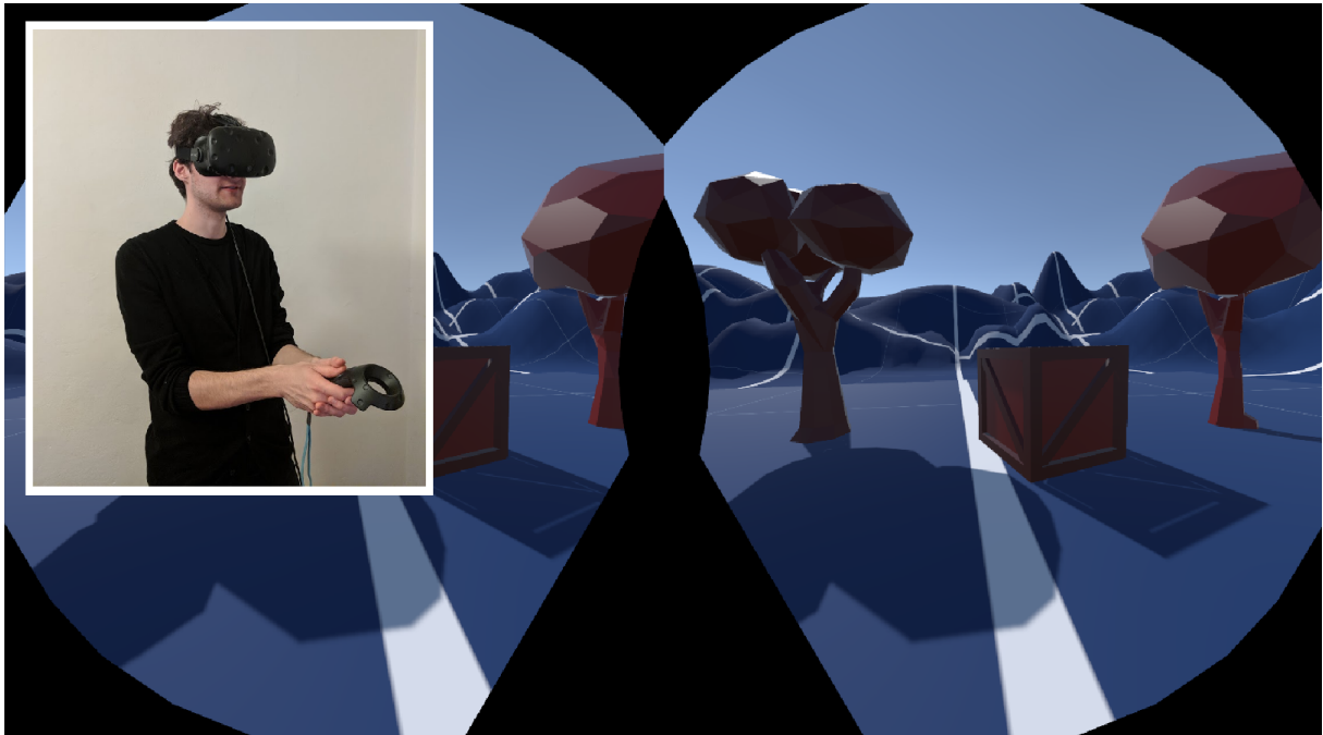
Figure 3.8: The participants were equipped with the HTC Vive headset and its 6DoF hand controller.
