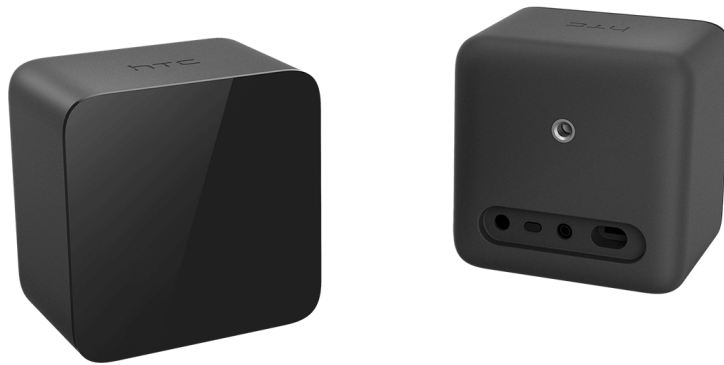
Figure 2.6: The Vive Base Stations: laser-based tracking system (image source: [18]).
